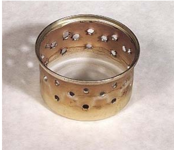
Vent holes made with an awl before flattening the collars (+)
