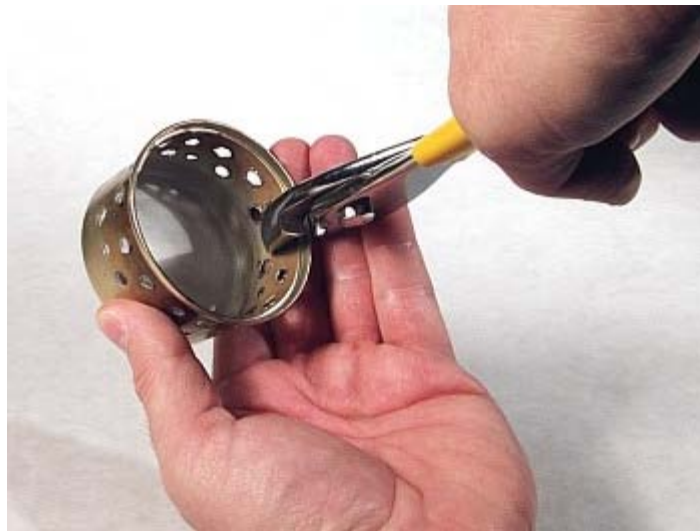
Flattening vent hole collars (+)
