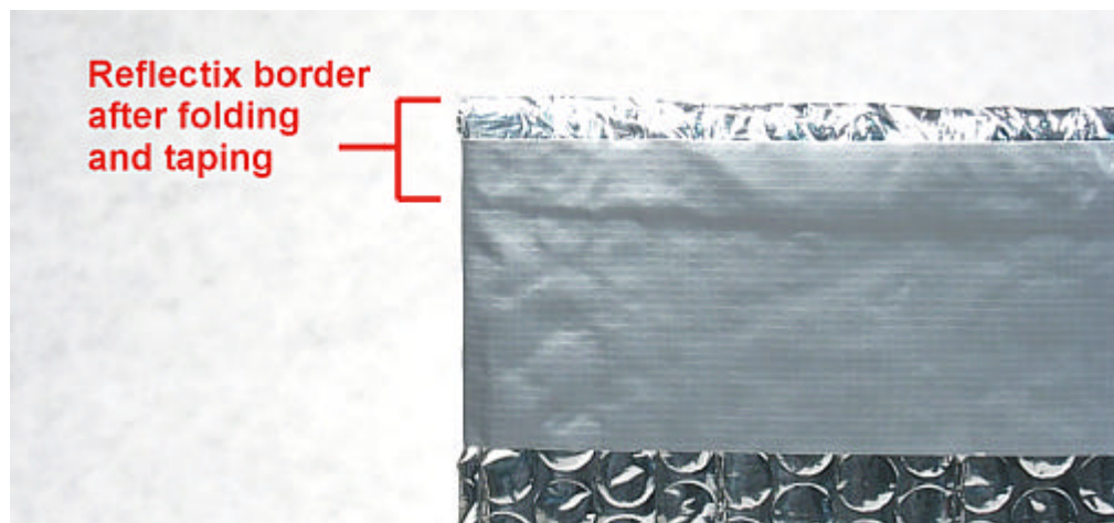
This edge now becomes the top of the cozy (taped surface goes inside) (+)
