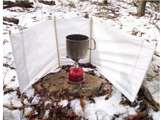
Tyvek KiteScreen supported with wooden dowels (+)
