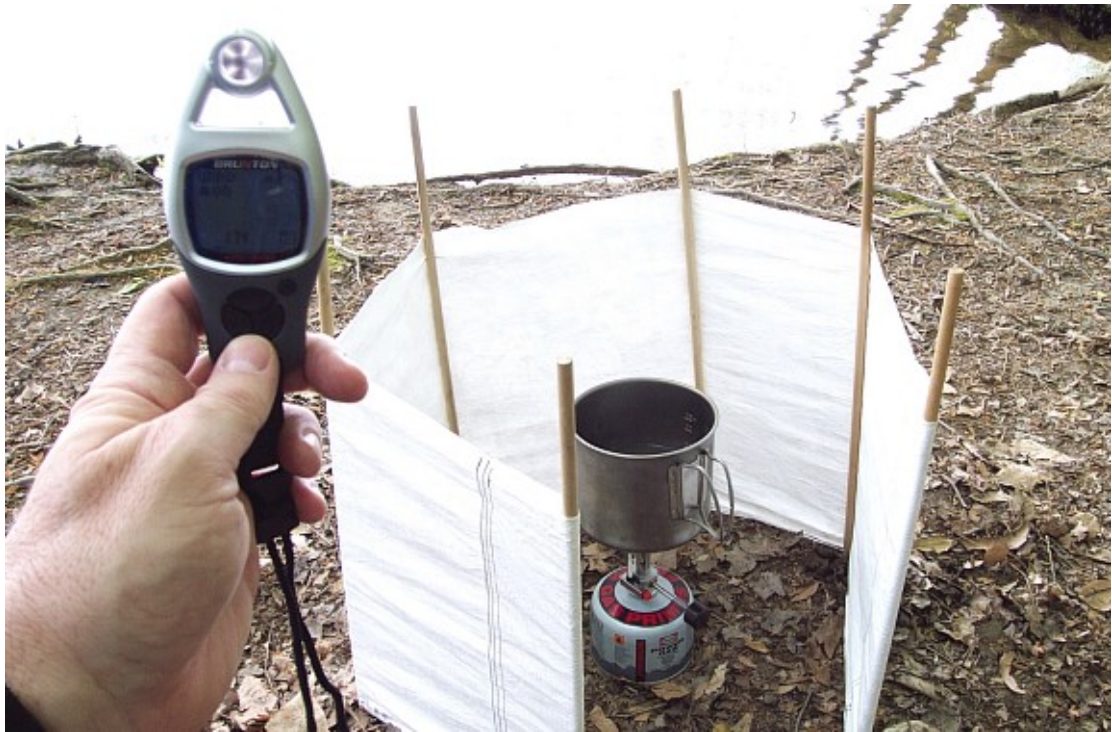
Measuring wind speed using a Brunton anemometer (wind meter) (+)
