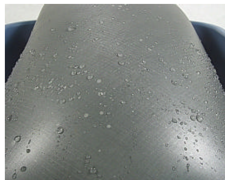
Close-up of water leaking through the silnylon fabric (+)
